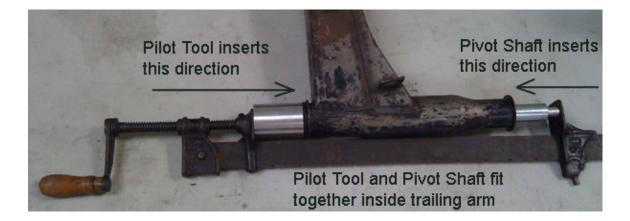
2 – Remove the rubber bushings and pivot shafts.
